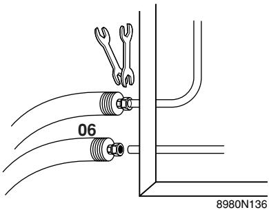
2. On the last panel of a panel group, the integrated return pipe is connected to the panel's serpentine piping. The return pipe link (50) is connected across the pipe connections of the solar panel. Remove the plastic dust caps from the pipe connections and fit the clamping ring fittings (11) onto the panel's pipe connections.
