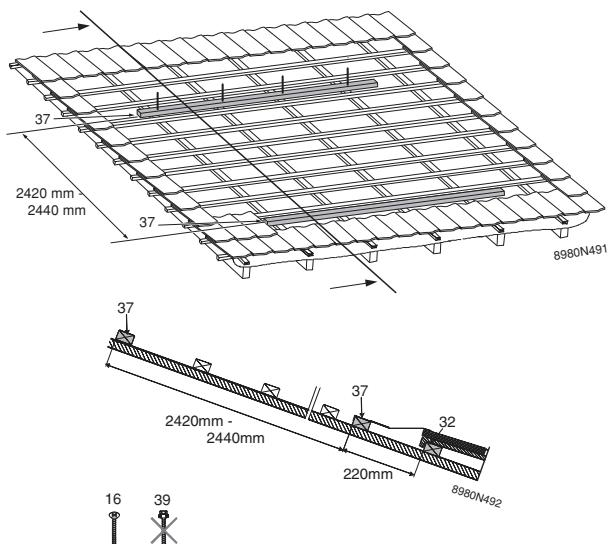
4. Place the **left** bottom cover plate (36-A) flush left on the horizontal fixing batten (37) and slide it downwards so that its top lip is seated against the fixing batten (37).
