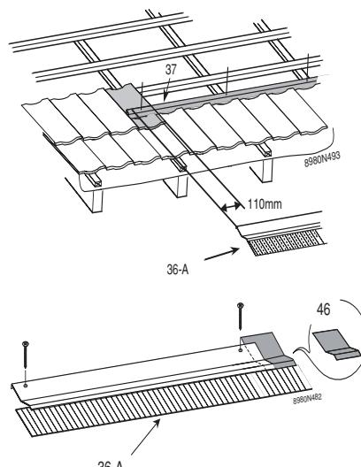
6. Check the position of the lower left cover plate and fix it to the fixing batten (37) using a second 3,9 x 25 mm screw (45).
